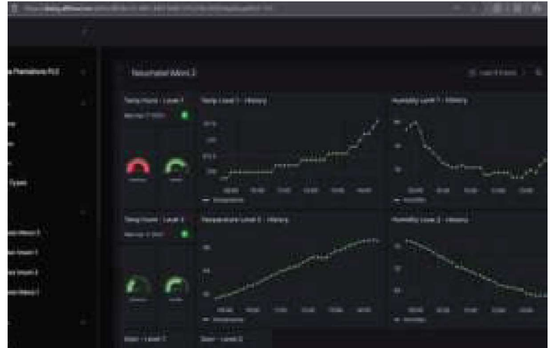
IoT Temperature Monitoring System for Drying Towers
